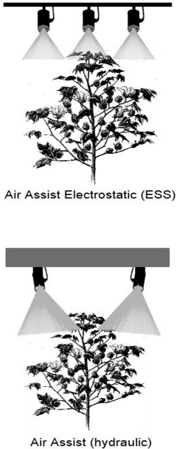
Fig. 2. Sprayer nozzle arrangement and spray direction for the air-assisted sprayers.
